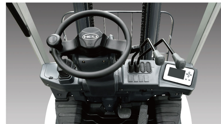
IC truck type control valve stem, better fit to the driver's habits
